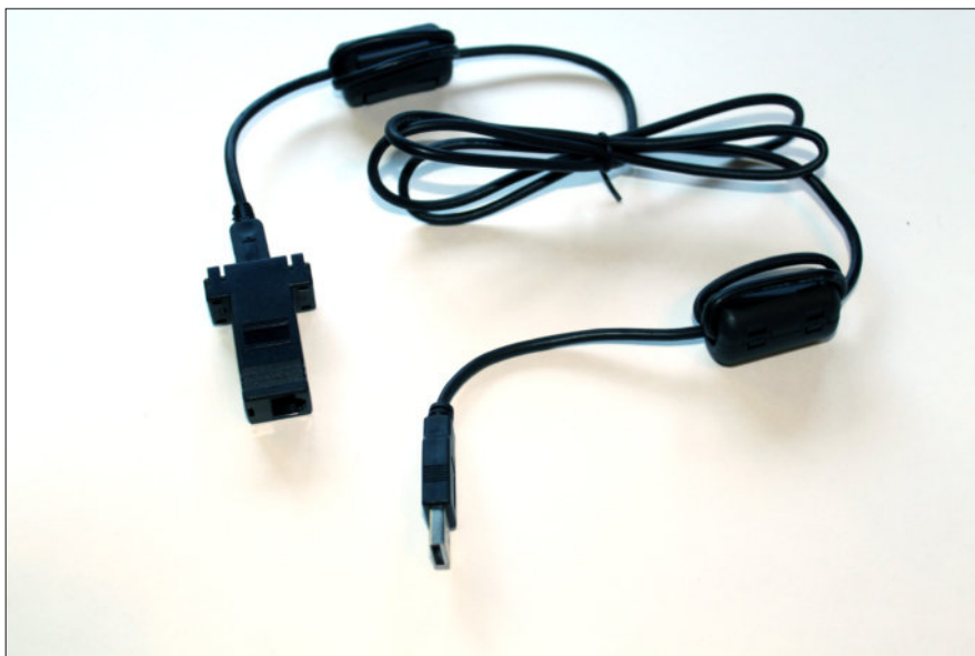
Figure 3-4: A USB adapter converts the RS-485 protocol required by the ShowTime PC controller to USB.
