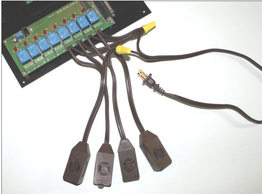
Figure 1-11: The main controller board with the line voltage wiring in place.
