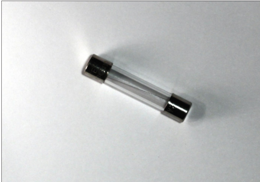
Figure 2-6: A 2 A, 1-1/4" x 1/4" AGC fuse.
