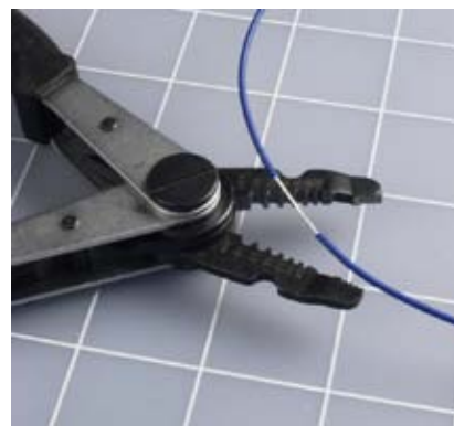
Figure 5-61. Wire strippers expose the solid conductor at intervals along a 22-gauge wire.
