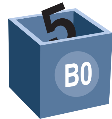
Figure 5-141. To understand how a program works, visualize a variable as being like a “memory box” with its name on the outside and a number stored on the inside.
