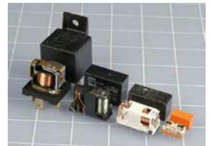
Figure 2-57. Four assorted 12-volt relays, shown with and without their packages. The automotive relay (far left) is the simplest and easiest to understand, because it is designed without much concern for the size of the package. Smaller relays are more ingeniously designed, more complex, and more difficult to figure out. Usually, but not always, a smaller relay is designed to switch less current than a larger one.
