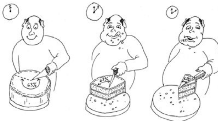
Figure 2-81. If our gourmet always eats just 63% of the cake still on the plate, he "charges up" his stomach in the same way that a capacitor charges itself. No matter how long he keeps at it, his stomach is never completely filled.
