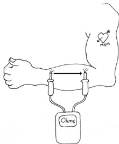
Figure 1-29. Moisten your skin before trying to measure its resistance. You should find that the resistance goes up as you move the meter probes farther apart. The resistance is proportional to the distance.
