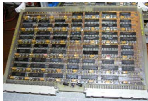
Figure 4-65. Hobbyist Bill Buzbee built himself a web server entirely from 7400 series logic chips, the oldest of which was fabricated back in 1969. The web server can be found online at http://magic-1.org , displaying pictures of itself and details of its construction. The picture here that Bill took shows just one of the circuit boards of this remarkable project.
