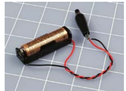
Figure 1-32. Shorting out an alkaline battery can be safe if you follow the directions precisely. Even so, the battery is liable to become too hot to touch comfortably. Don't try this with any type of rechargeable battery.
