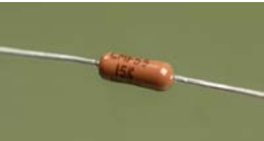
Figure 1-41. Some modern resistors have their values printed on them, although you may need a magnifier to read them. This 15K resistor is less than half an inch long.
