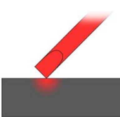
Figure 3-45. With only a small surface area of contact between the iron and the working surface, an insufficient amount of heat is transferred.
