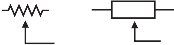
Figure 2-42. Potentiometer symbols: the left is traditional and used in the United States, the right is European. In both cases the arrow indicates the wiper (usually the center terminal).
