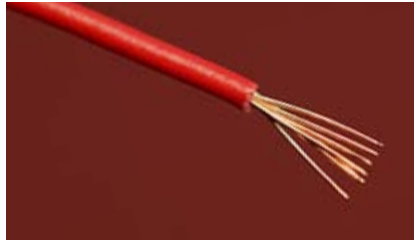
Figure 2-8. Stranded is more flexible, but cannot be used easily with breadboards.
