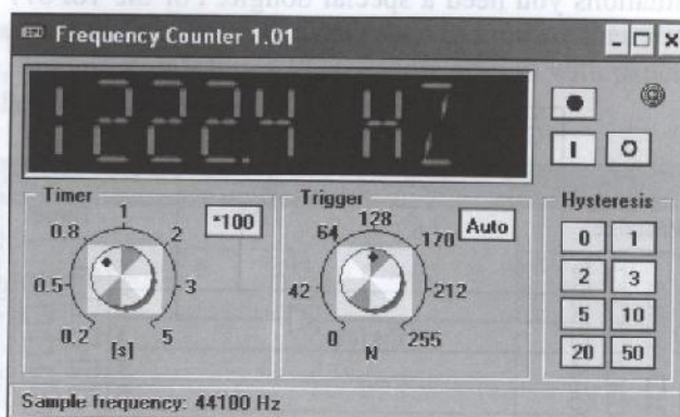
Figure 15. Software frequency counter.
