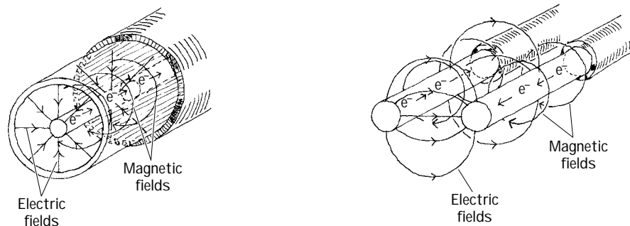
FIGURE 3.9 Illustration of the electrical and magnetic fields within a coaxial and paired cable.
