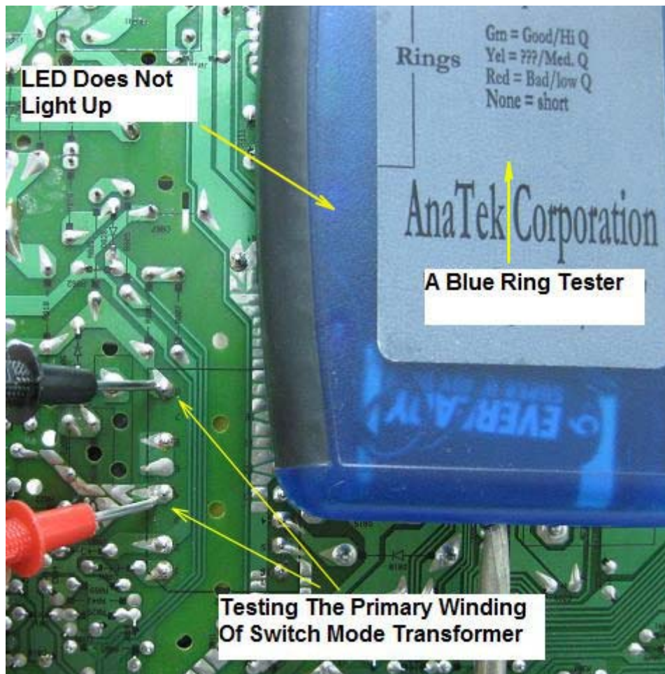
Figure 18.12- This Is The Right Way To Test SMPS Transformer Primary Winding
