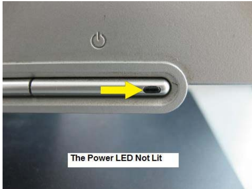
Figure 9.1- The LED Act As A Power Indicator
