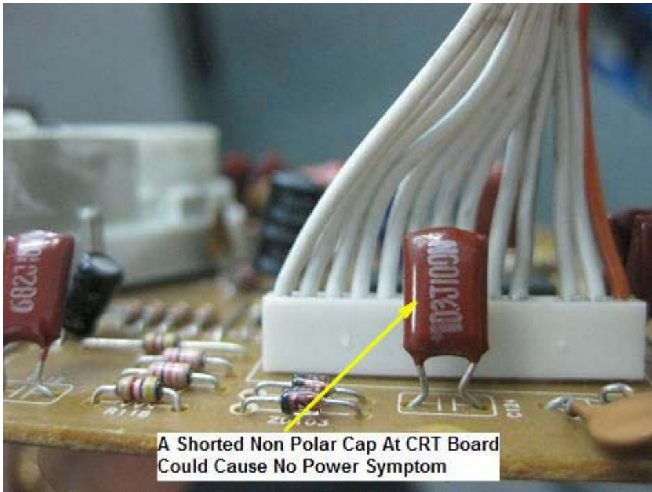
Figure 18.1- Shorted Non Polar Capacitor At CRT Board
