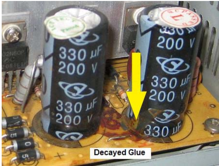
Figure 20.4- Decayed Glue Found In ATX Power Supplies
