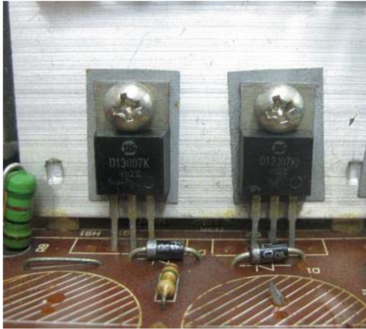
Figure 20.1- Power Transistors In ATX Power Supply
