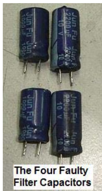
Figure 20.8- The Four Faulty Filter Capacitors
