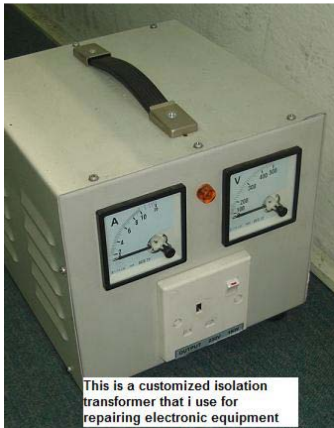
Figure 8.5- An Isolation Transformer
