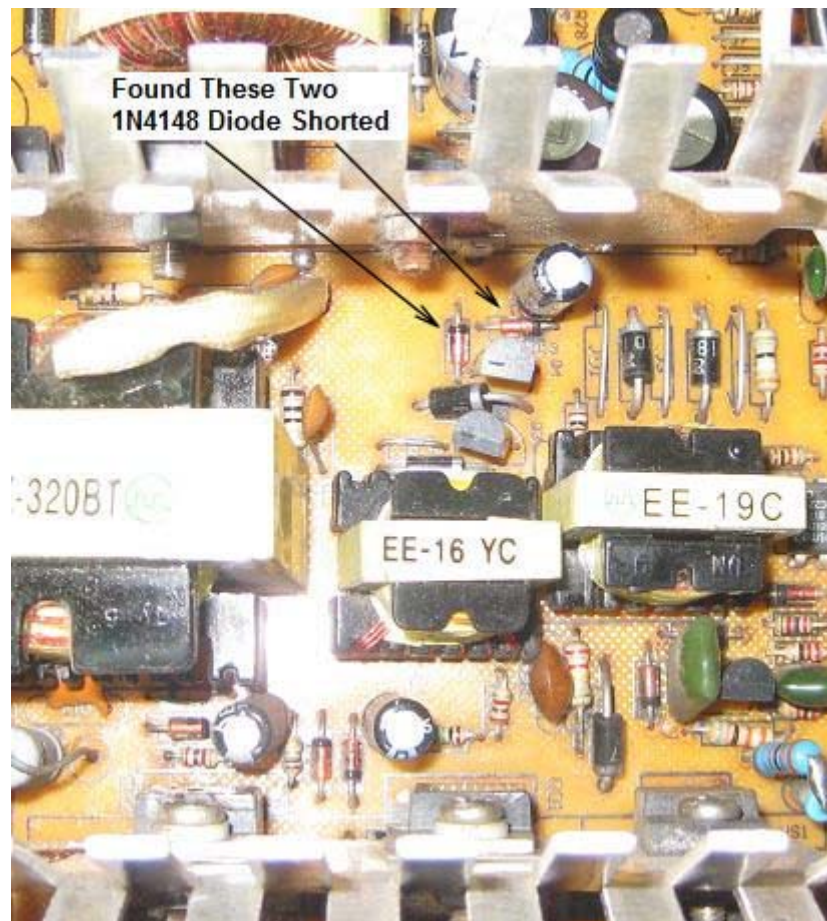
Figure 20.11- Low Output Voltages Could Be Caused By Shorted Signal Diodes In The Secondary Side
