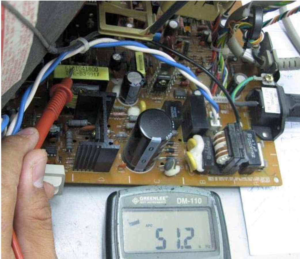
Figure 12.19- The Right Way To Place Your Test Probe On The SMPS Transformer
