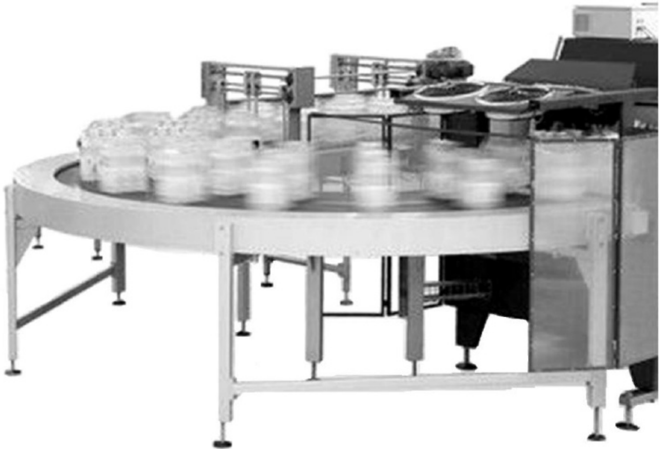
Figure 8.41: Bottle conveyor system The ladder logic program is shown in figure 8.42.
