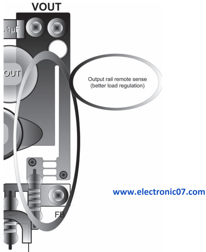
Figure 6-13 Output Sensed Remotely for Better Regulation
